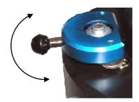
1. Turn the lever to the right: The watch dives into the water. The pressure in the cylinder. decreases and the leak becomes visible (Air-bubbles).
